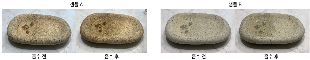
<Figure 7> Appearance of Samples A and B before and after Absorption
